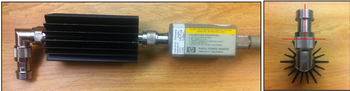
NOTE: Ensure the adapter is positioned perpendicular to a flat side of the attenuator heatsink:
